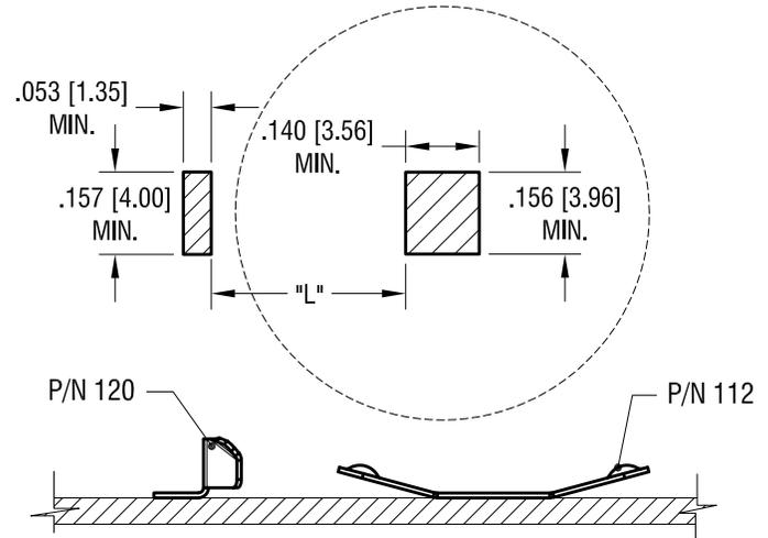
MTG LAY OUT WHEN USE WITH P/N 112
