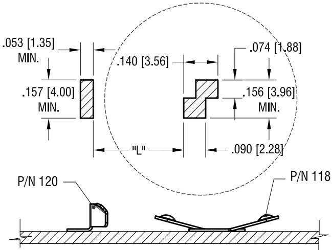
MTG LAY OUT WHEN USE WITH P/N 118
